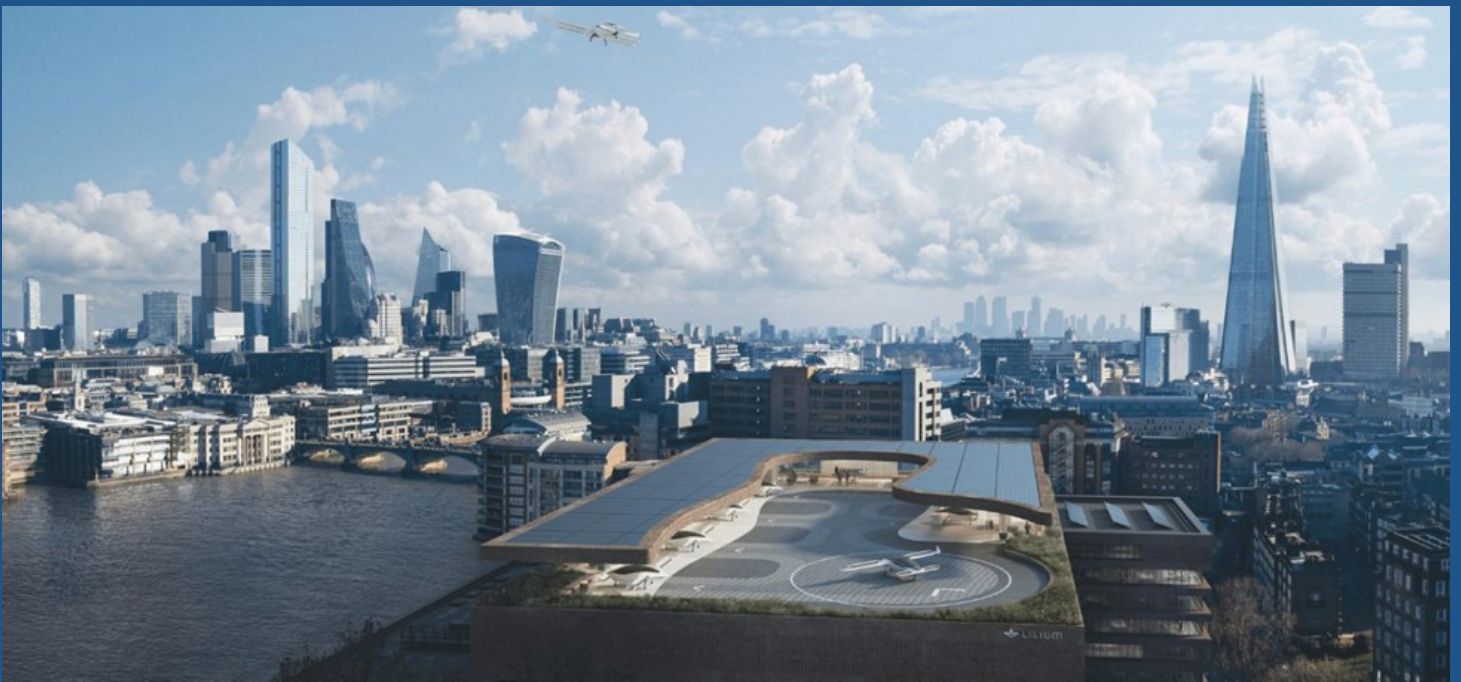
Figure 10 - As passenger-carrying AAM aircraft emerge and become certified for operation above cities and regions, on-demand air taxi concepts will take hold. The aircraft will need landing pads called “vertiports” sited at convenient locations such as airports, hospitals, downtown, atop parking garages, major trucking and distribution companies, and headquarters of large corporations.
